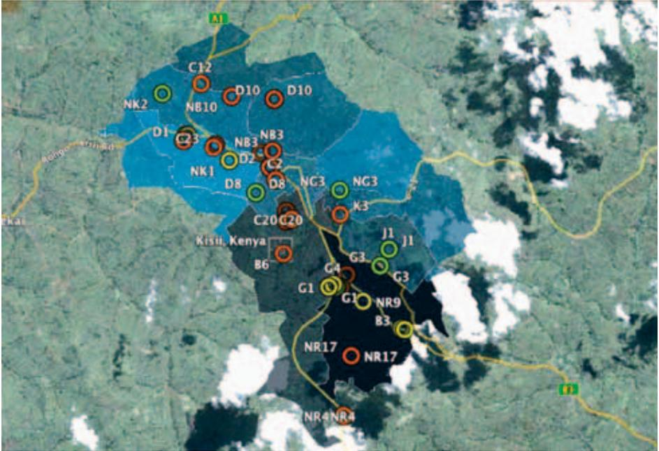
**Figure 8:** Geo-referenced water quality data collected using the tests in Kisii (July 2010) and represented on an online mapping tool (green = low risk, yellow = moderate risk, orange = high risk). Photo © 2010 Google
